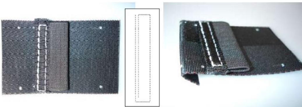
2.5 Stitch Elastic Keeper onto TYPE 12 Webbing as shown. Use Nylon E Thread
