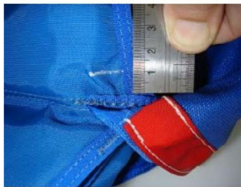
4.9 Mark 10mm along Flap #1 from intersection as shown
