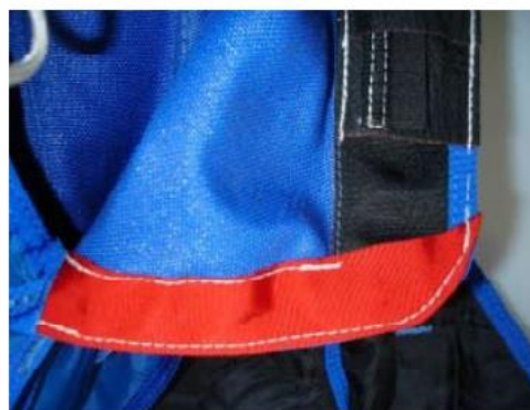
4.5 Finish Tunnel as shown. Backtack at least 10mm
