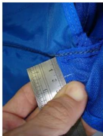
4.2 Measure and mark 20mm from Intersection between Flap #1 and Flap #2. This mark is the alignment mark for the start of the tunnel
