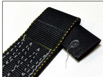
Fold in sides of riser to allow installation of #6 Rapide link
