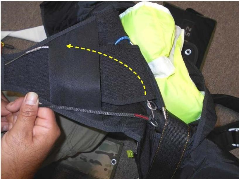
Pass the Ripcord cable and the Top Reserve Closing Flap under the T-IV retaining webbing.
