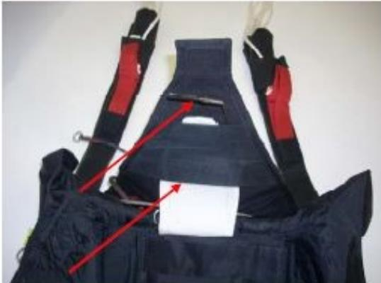
Before proceeding check to be sure that the Top Closing Flap and the Ripcord is under the tape of the Top Cover Flap.
