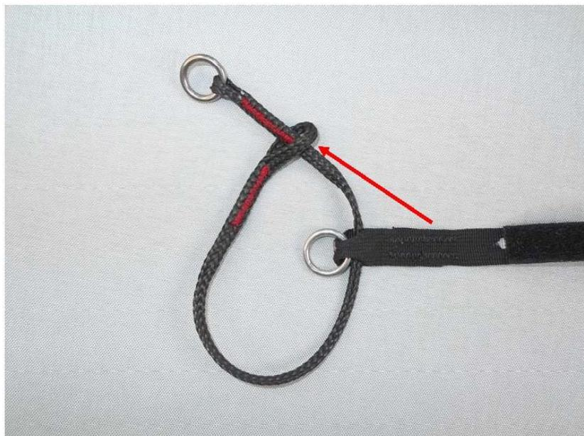
Pass the mini ring of the HMA line through the loop on the end of the "Reserve Boost" lanyard.
