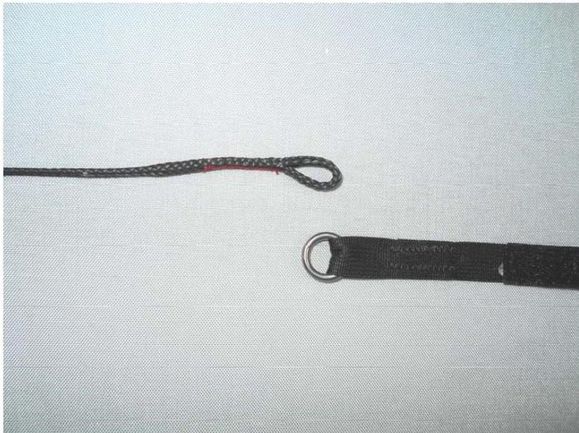
Remove HMA line from the mini ring.
