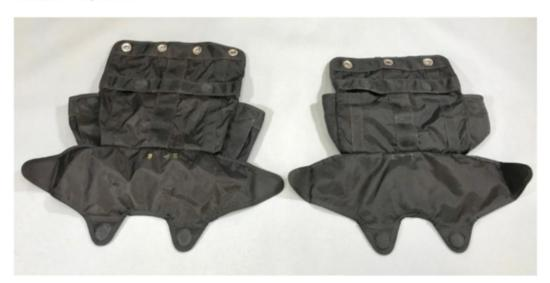
This bulletin **does not** affect the semi-stowless deployment bags delivered after Nov. 1<sup>st,</sup> 2017, which have red stow pockets for the magnetic mouth closure system.
