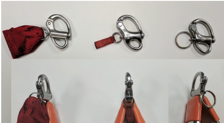
Wichard Shackle- Marked with "W" Half hinge design
