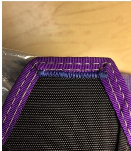
Open up the pin protector flap and place the tip under the foot of the sewing machine (para - pack side up). Run a zig zag stitch across the end portion (approx. 4mm wide) with a throw being each side of the edge of the binding tape, (i.e. binding tape edge runs in center of the stitch). Put a small back tack at the beginning and end of the line of zigzag stitching. Trim thread and inspect. The end result should resemble above picture.
