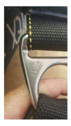
These DO form part of the recall and are in addition to the ones referenced in the original Bulletin (PSB#2016-01) stamped "DSF".
