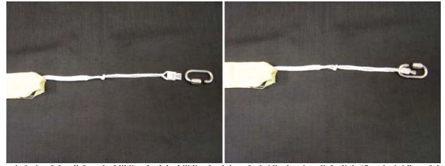
After you larks head the slink to the kill line feed the kill line back into the bridle then install the link #5 to the bridle and the Slink.
