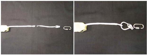
First Extract the kill line out of the bottom of the drogue bridle, remove the Link #5 and larkshead the slink to the end of the kill line
