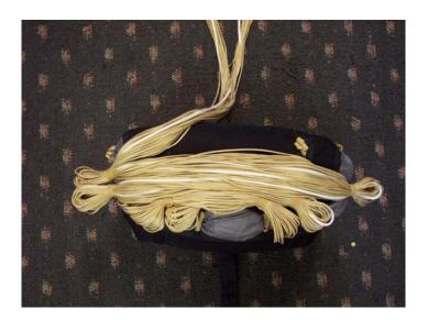
2. Separate the line groups into a left and right riser group and place these lines into the next stow on the same side of the deployment bag, leaving approximately 12-15 inches of excess between the last stow and the risers.
