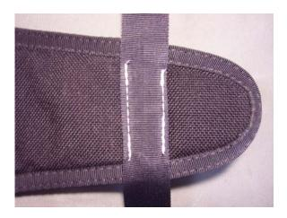
7. Cut the Type 3 tape to leave approximately 1" tails. Roll the tails to hide any exposed edges and sew the tails to the binding tape.
