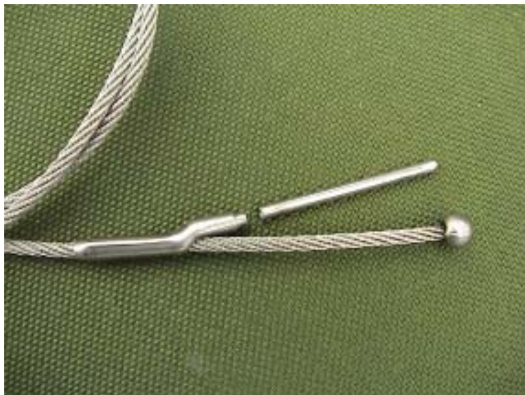
Broken Ripcord Pin
