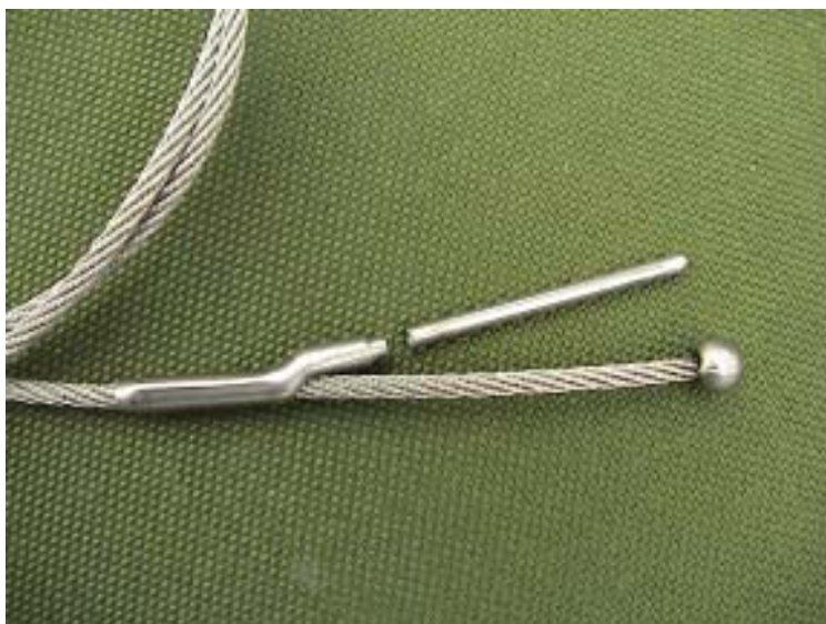
Broken Ripcord Pin
